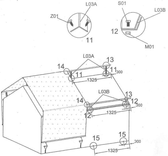
At the base of the Greenhouse place a W01 300mm from the back of the Greenhouse and place another at 1325mm. Predrill the holes using a 6mm diameter drill and screw fix the brackets in place being careful not to over tighten. Repeat the process on the opposite side of Greenhouse.
