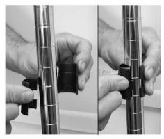
3. Snap the sleeves into the post groove. Sleeves must be snapped together with the small tapered side facing up.
