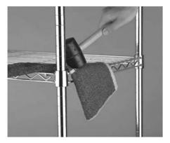
7. Pushing firmly down on every shelf at corners by rubber mallet to secure the shelf in a place over the sleeves. (Using a rubber mallet can make installation easier-use caution not to damage the unit).
