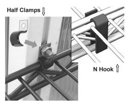
Locate the bench fasteners. They can be installed after the benches have been assembled. The half clamps are used to secure the bench to a wall, and the N hooks are used to fasten multiple benches together or as hangers. There should be 2 half clamps and 2 N hooks per bench.
