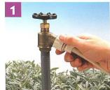
Push and twist the long section of tubing into the water hose adapter about 1". Then pull on the tubing to make sure it is snug, and attach it to a faucet or water hose. The screen in the adapter should be curved away from the tubing inside.
